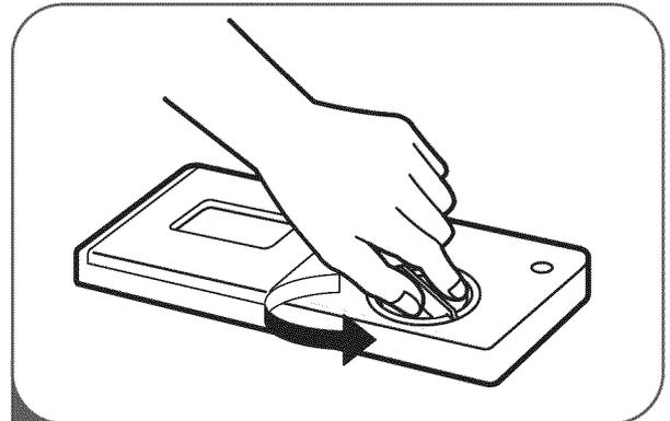
**1** Rotate the round cap counterclockwise to remove it.
