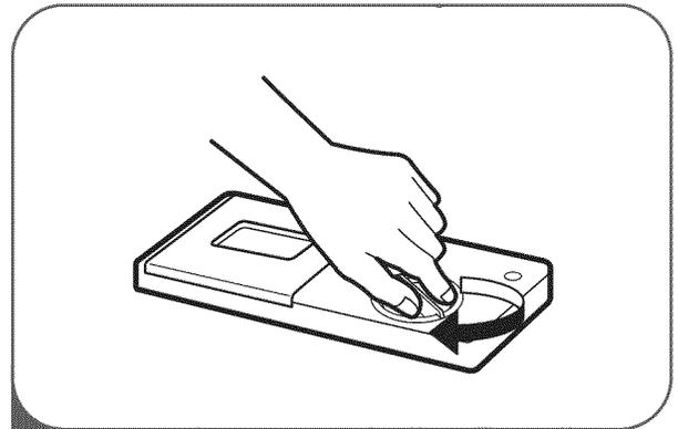
**3** Replace the cap and turn clockwise to lock. Rinse aid will be dispensed automatically during the final rinse cycle.
